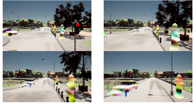
Fig. A.3: Sample renderings of the left turn trajectory with the adversarial perturbations in CARLA from the ego vehicle's point of view. Four different snapshots from the evolution of the trajectory are shown.
